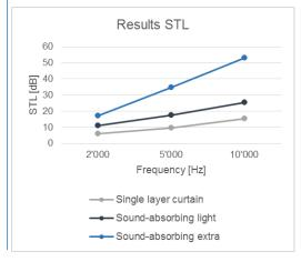
The results show the better performance of soundabsorbing curtains due to the higher area weight and higher airflow resistivity compared to the single layer curtains. To better reduce galley noise intrusion into the passenger cabin Lantal recommends sound-absorbing curtains.
