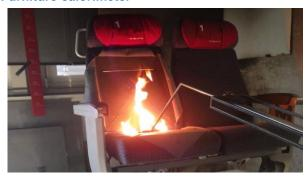
The test is performed according to EN 45545-2 Annex B in the furniture calorimeter pursuant to ISO 9705.
