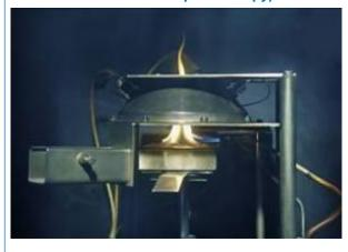
This test analyzes the smoke density and smoke toxicity potential of combustible materials and components.
