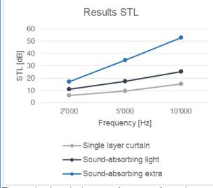
The results show the better performance of soundabsorbing curtains due to the higher area weight and higher airflow resistivity compared to the single layer curtains. To better reduce galley noise intrusion into the passenger cabin Lantal recommends sound-absorbing curtains.
